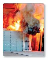
While solidly grounded systems are an improvement over ungrounded systems, and speed the location of faults, they lack the current limiting ability of resistance grounding and the extra protection this provides. The destructive nature of arcing ground faults in solidly grounded systems is well known and documented and are caused by the energy dissipated in the fault.
