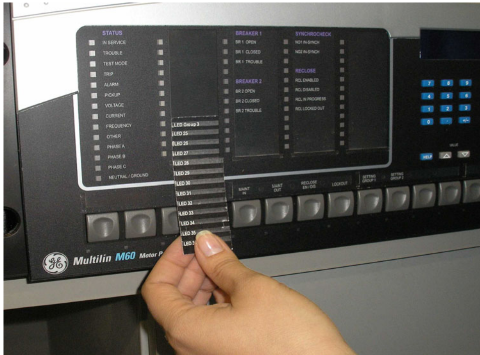
Figure 4-16: STEP 7 - SLIDE HALF OF THE PRINTED LED LABEL INSIDE THE POCKET
