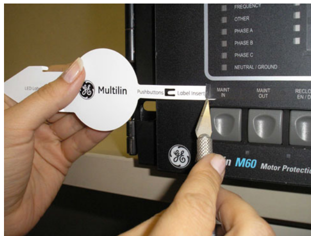
Figure 4-19: STEP 1 - USE KNIFE TO LIFT THE PUSHBUTTON LABEL AND SLIDE TAIL OF THE LABEL TOOL UNDERNEATH. MAKE SURE THE BENDED TAB IS POINTING OUTWARDS ( IE - AWAY FROM YOU).
