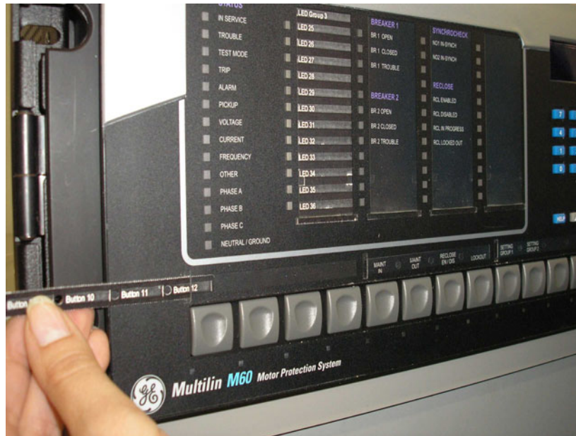
Figure 4-22: STEP 4 - SLIDE IN THE CUSTOM BUTTON LABEL AS SHOWN
