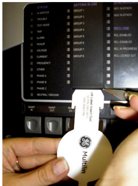
Figure 4-13: STEP 1 - USE KNIFE TO LIFT THE LED LABEL AND SLIDE THE LABEL TOOL UNDERNEATH. MAKE SURE THE BENDED UPPER TABS ARE POINTING OUTWARDS ( IE - AWAY FROM YOU).
