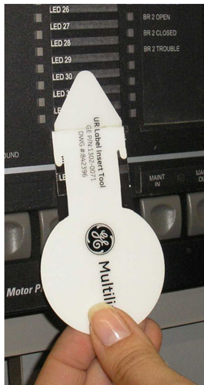
Figure 4-17: STEP 8 - SLIDE THE LABEL TOOL INSIDE THE POCKET AS SHOWN
