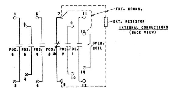
\*Figure 3 (0418A0799, Sh.1,bottom [8]) Internal Connections for HFA153K Relay (Back View)
