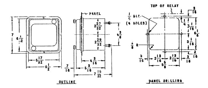
\*Figure 4 (0418A0799, Sh.1, top [8]) Outline and Panel Drilling Dimensions for HFA153K Relay for Semi-flush Mounting
