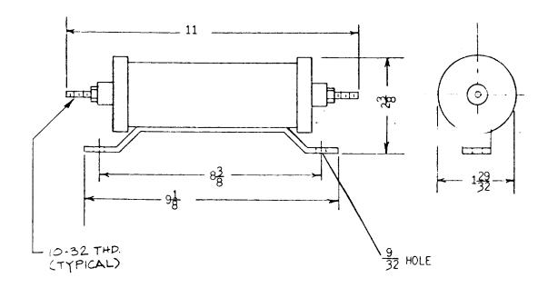
\* Figure 6 (0389A0752 [2]) Outline of External Resistor used with HFA153K Relays
