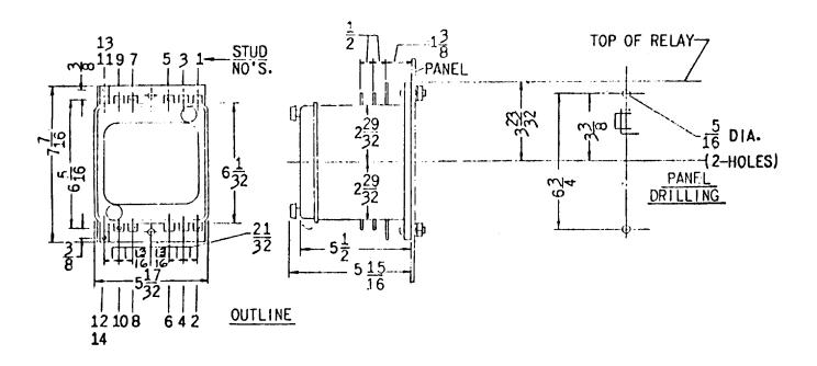
Figure 5 (0104A8527, Sh.1 [5]) Outline and Panel Drilling Dimensions for HFA153K Relays for Surface Mounting, Front Connected
