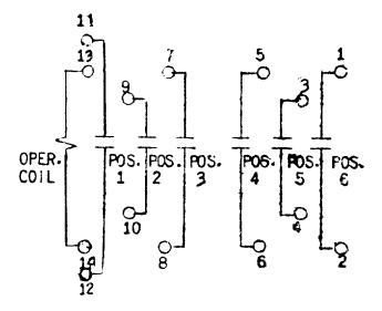
Figure 4 (0104A8526-7) Internal-Connections Diagram for HFA151 Relays (Front View)
