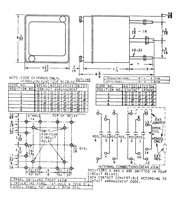
Figure 6 (K-6178931-12) Outline and Panel Drilling for Surface-mounted Type HFA151 Relay
