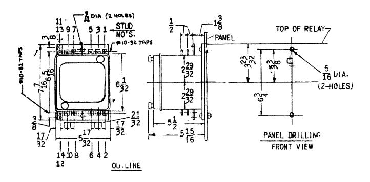
Figure 7 (0104A8526-7) Outline and Panel Drilling for Front-Connected Type-HFA151 Relay
