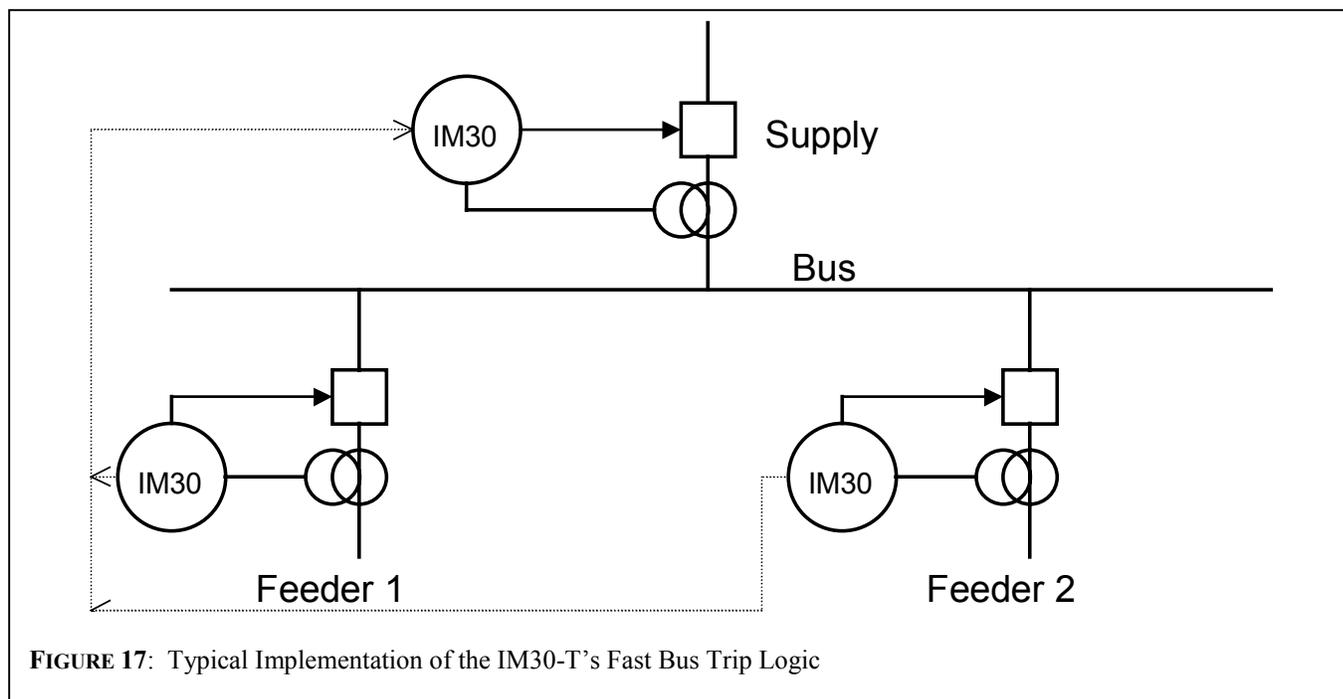
Figure 17 indicates typical application. It is assumed that all relays are set for both phase and ground overcurrent protection. In addition, it is assumed that both low and high set protective elements for both phase and ground elements are used. This document should be considered a guide as to the general methodology required to implement the described functions. It is incumbent upon the user to modify the described procedure as required for any given protective application.
