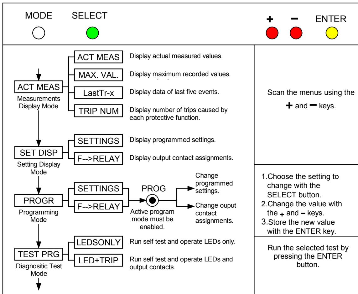
Figure 19: KEYBOARD FUNCTIONAL DIAGRAM
