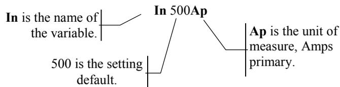
Table 2 details all of the relay setting variables. Please note that Dis indicates that this particular function can be disabled by entering Dis as the setting value.
