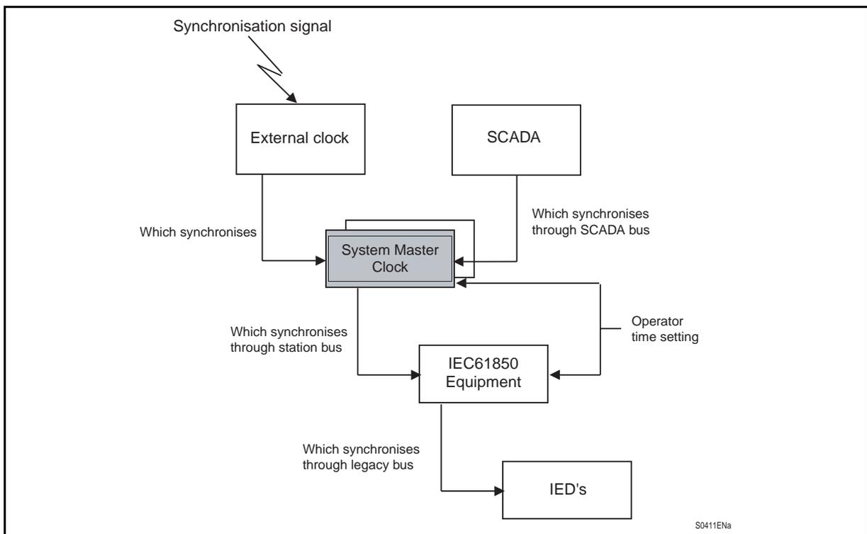
In case that external clock does not exist or is lost, the master clock equipment can be synchronised by a SCADA (only if the Master Clock computer manages a SCADA protocol) or by an operator. Synchronisation priority of the System Master Clock is in the following order:
