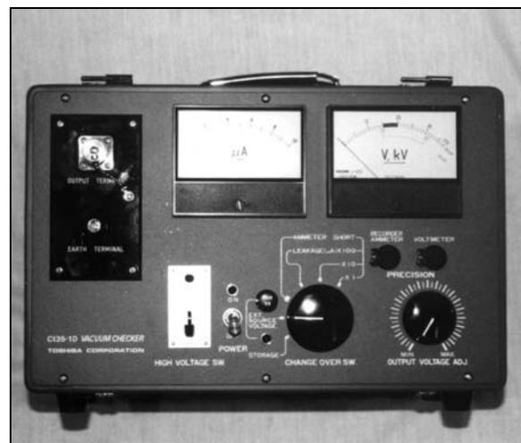
**Figure 11 - Toshiba Portable Vacuum Checker**
