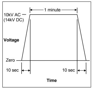
Figure 12 - Application of Test Voltage for Vacuum Check
