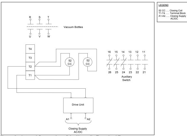
Figure 8 – Internal Connection of the Normally Energized Type
