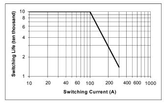
Figure 14 - Capacitor Switching Life
