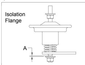
Figure 13 - Gap Measurement
