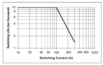
Figure 14 - Capacitor Switching Life
