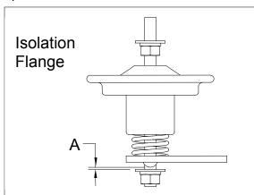
Figure 13 - Gap Measurement
