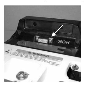
Figure 8 – Control Terminals Location
