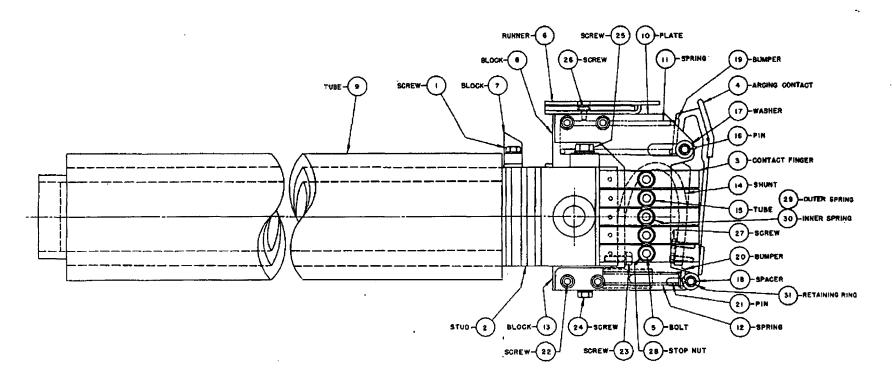
FIG. 24 TYPICAL TOP BUSHING ASSEMBLY APRIL 28, 1960 71-401-252
