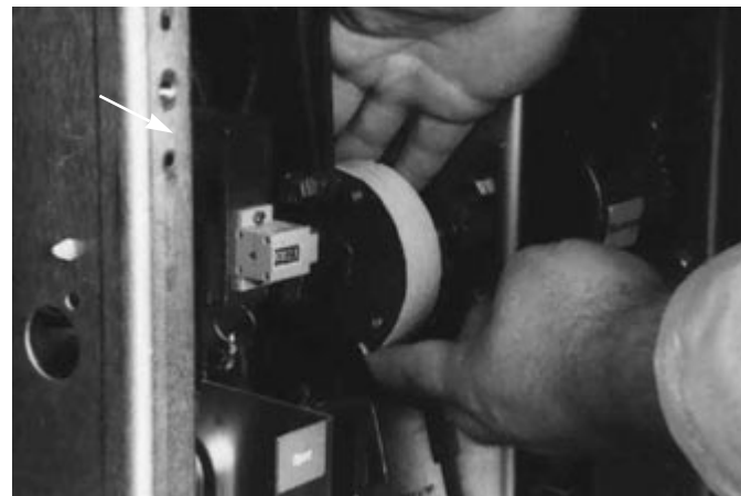
Figure 6-8 Attaching Tape Around to Back of Cam
