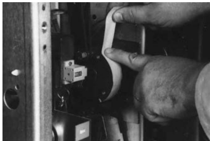
Figure 6-7 Wrapping Tape Up Around Cam
