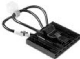
**NOTE: For RMS/R 510 Basic Kits, the External Harness is the plug pictured above. It is to be plugged into the right side of the Trip Unit.**
