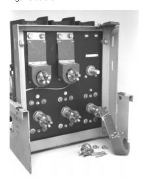
Step 4: Installing the Retrofit Components on the Trip Unit Mounting Platform
