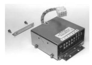
B. Mount the Trip Unit Mounting Brackets to the Trip Unit, as shown, using the (2) .190-32 x 4.00" screws, (2) lock washers, (4) flat washers, and (2) nuts supplied. Note the Mounting Brackets are to be installed with the holes towards the bottom of the Trip Unit. Also note that the screws, with flat washers installed, are inserted from the bottom of the Trip Unit and the flat washers, lock washers, and nuts are installed from the top.
