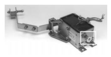
NOTE: Loc-Tite<sup>®</sup> 242 will be applied to the threads on the end of the DTA Shaft to secure the Flange Nut when final adjustment is made later in the Retrofit process.
