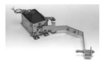
NOTE: Loc-Tite<sup>®</sup> 242 should be applied to the threads of all screws and bolts used to assemble and mount the DTA Assembly.
