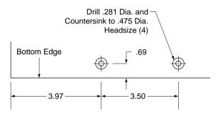
Right Side of Breaker Shown – Drill Both Sides (11.50" High Side Frame Rail)
