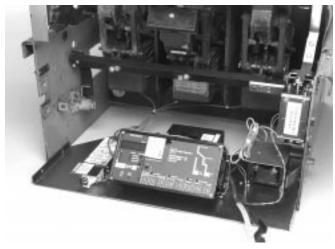
Step 6: Assembling the Direct Trip Actuator (DTA) Assembly
