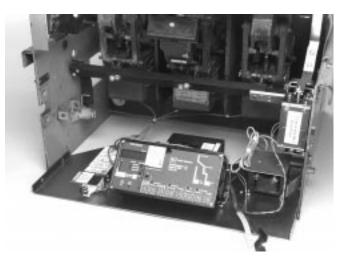
A. Align the holes in the Breaker Mounted CPT with the predrilled holes in the Trip Unit Mounting Platform, as shown, then secure
