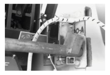
B. The DTA reset adjustment is achieved by turning the flange nut on top of the DTA shaft. If adjustment is required, remove the flange nut from the DTA shaft and apply Loc-Tite<sup>®</sup> 242 to the shaft threads. Then screw the nut onto the shaft, adjusting the gap to .19" - .25" as shown.
