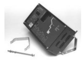
C. Remove the Trip Unit Cover and install the Rating Plug. Replace the cover.
