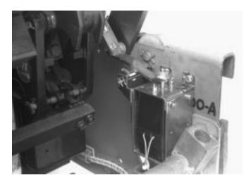
A. Align the holes in the DTA Mounting Brackets with the holes drilled in the right Breaker Frame in Step 8. Mount the DTA Assembly to the right Breaker Frame, as shown, using the (4) .190-32 x .625" screws, (8) flat washers, (4) lock washers, and (4) nuts supplied. When positioning the DTA Assembly, assure that the Reset Lever is behind the Striker Plate.
