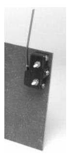
Step 8: Drilling the Mounting Holes in the Breaker Frame
