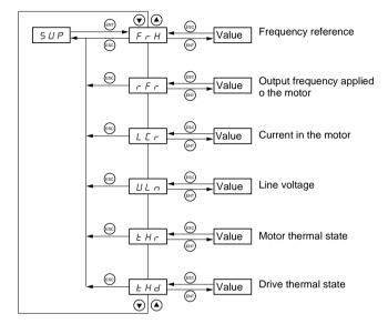
When the drive controller is running, it displays the value of one of the monitoring parameters. The default display is frequency reference (parameter FrH).
