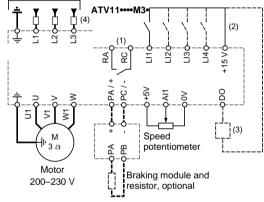
NOTE: The line supply terminals are shown at the top and the motor terminals are shown at the bottom. Connect the power terminals before connecting the control terminals. Install surge suppressors on all inductive circuits located near the drive controller or coupled to the same circuit.
